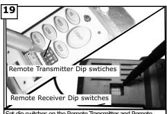
Set dip switches on the Remote Transmitter and Remote Receiver to the same settings. This must be done so the units will communate properly. If you have other fans you can set to control from one transmitter by setting both receivers the same as the transmitter. If you have more than one fan with remote. You can set the dip switches to different positiosns to have seperate control.
